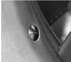
Measuring connector in inlet cone Hose pipe to connecting piece in the side wall Connecting piece (external diameter of 6mm) for the pressure measurement
