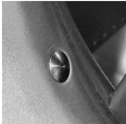
pressure tapplings in inlet cones
